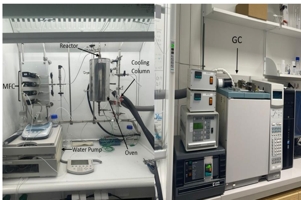
Figure 7: Experimental setup for evaluation of Cu modified ZSM-5, and SAPO zeolite catalysts in \text{N}_2\text{O} decomposition reaction.
