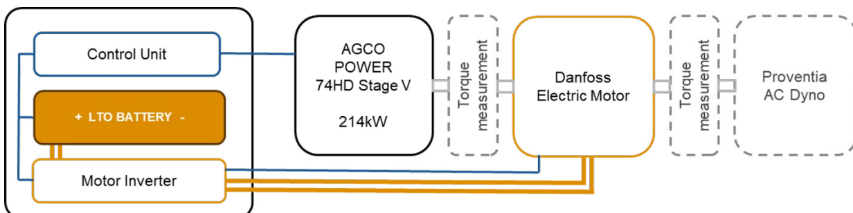
Figure 1. Hybrid system architecture at test laboratory
