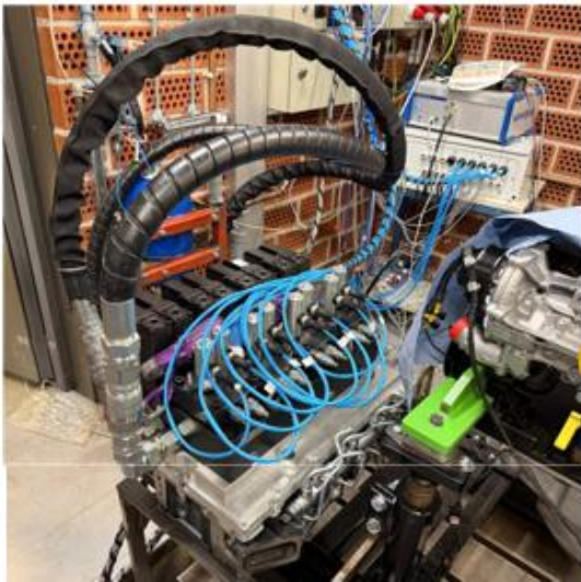
Figure 1. EHVA system under testing with cylinder head
