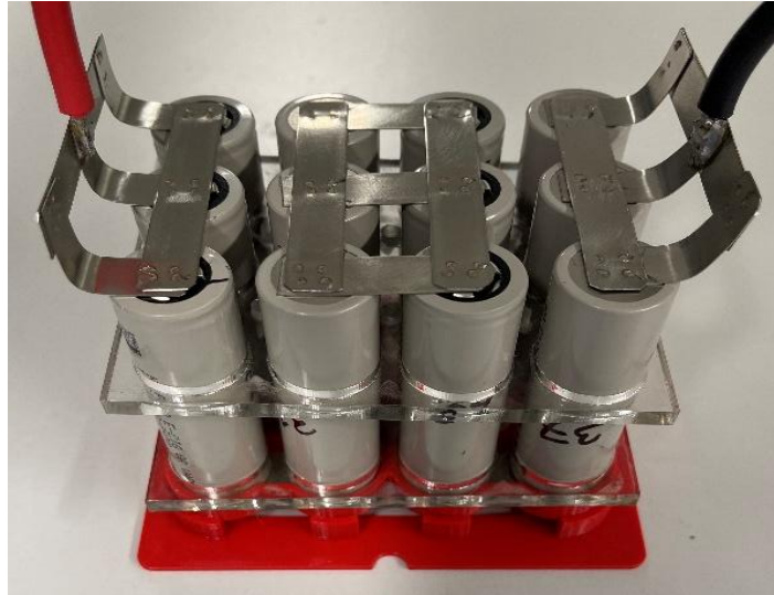
Figure 23 Battery Module Configured in a 3P4S Arrangement(Avik, 2024).
